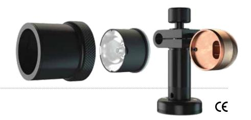
The luminaire is composed of: front aluminum module (1), LED with optical lens (2) and rear copper heat sink (3). The lighting fixture, in its versions, guarantees different power, beam spread, colour hues and two CRI options.
